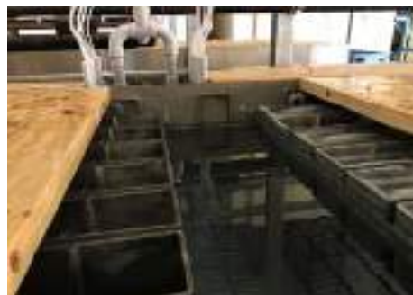
Stainless steel molds immersed in brine
