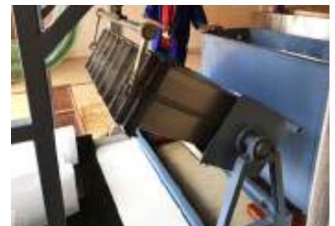
Overturning of the ready blocks
