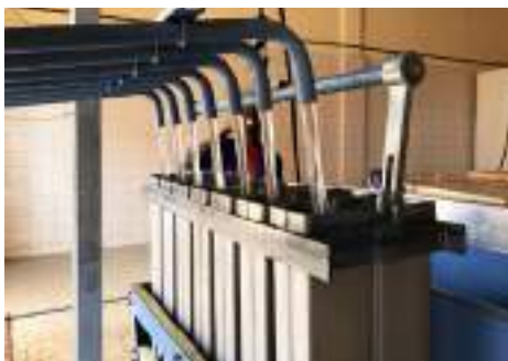
Filling phase of the moulds with water
