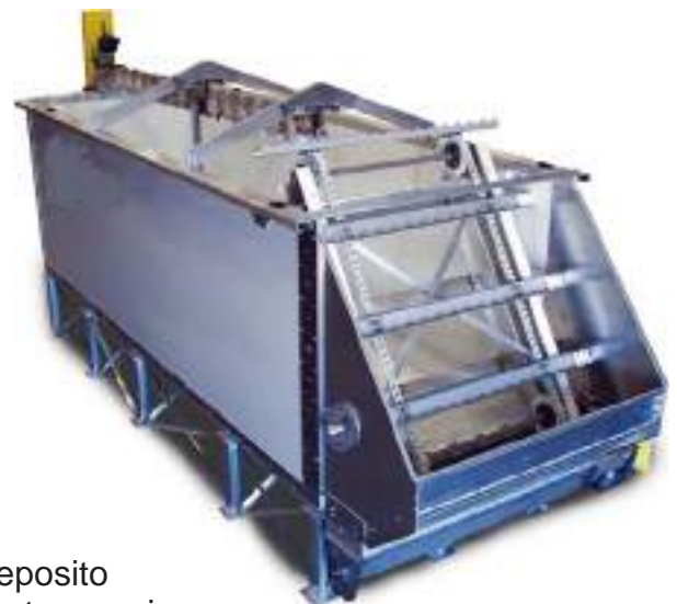
Ice storage deposit with walking floor and LIFO system: the mass of ice is transferred to a rake that erodes it
